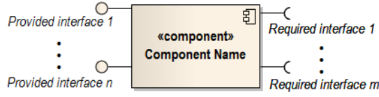
Figure 2. UML Graphic representation of a software component
